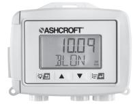
**BL OFF** will flash on the display when the Backlight function is being turned off. After a couple of seconds, the BL OFF message will disappear from the screen.
